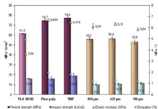
Figure 1. Mechanical properties of PLA 3051D composites with 30 wt% of two wood pulp types: pine and TMP and three wood flours with different particle sizes.
