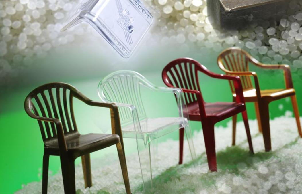
different material and processing approaches to improve the crystallinity of injection moulded PLA products. The effects of different nucleating agents as well as different PDLA types were studied, showing drastic improvements in crystallisation speeds. In profile extrusion, initial samples with foamed cores were produced by TCKT.
