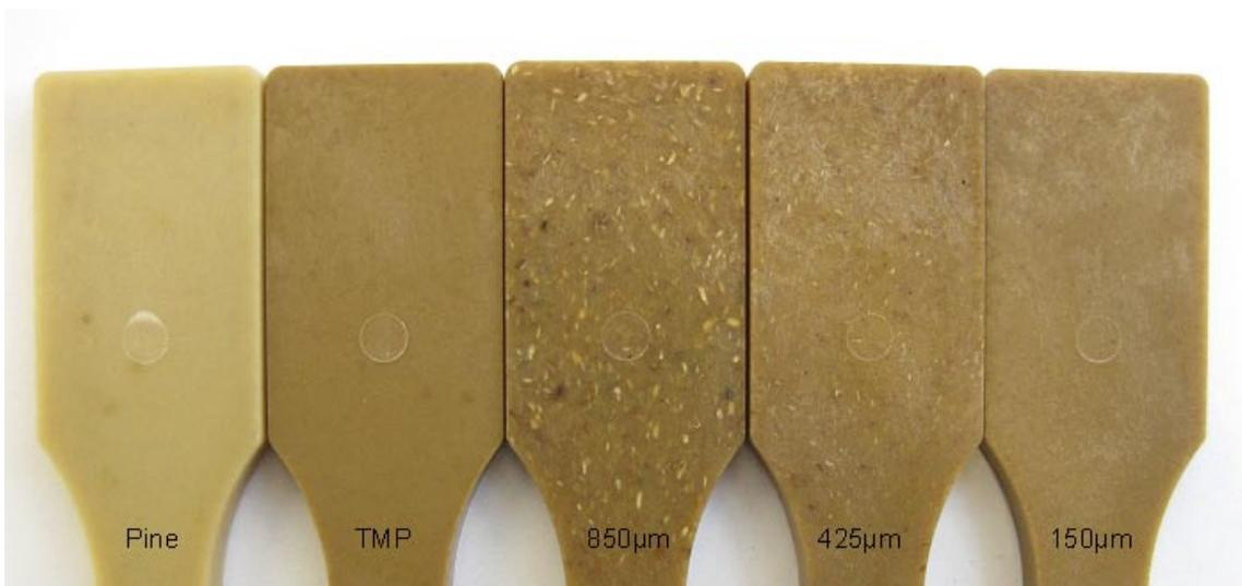
Figure 2. Macroscale fibre dispersion of pine pulp, TMP and three wood flours with different particle sizes in PLA matrix with fibre content of 30 wt-%
